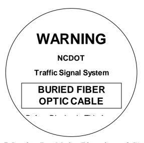
Overall Junction Box Marker Dimensions: 2.5" diameter Text: Black Background: Light Gray (to blend with concrete and granite surfaces)
